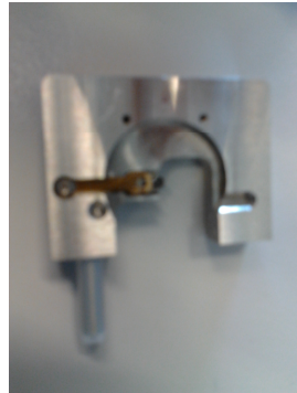
Figure 18: Cantilever holder with cantilever mounted.
